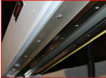
View showing precision ground replaceable track
